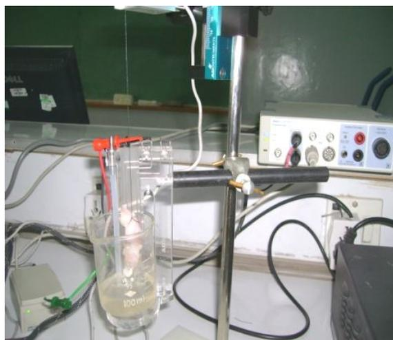
**Figure-2: Muscle setup on PowerLab<sup>®</sup>**
