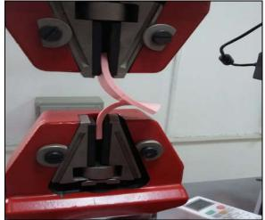
Figure-2: Tear strength testing with Universal Testing Machine
